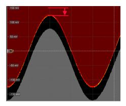
Figure 10-5: Waveform mask with vertical width = 0.5 div and vertical position = -0.5 div
