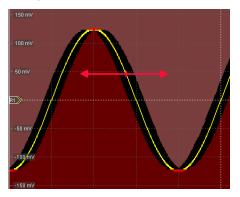
Figure 10-2: Waveform mask with horizontal width = 0.2 div
