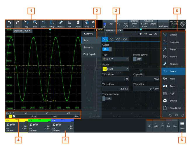
Figure 3-8: Control elements on the touchscreen
