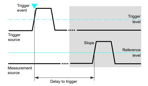
To configure the trigger conditions, use the trigger setup. To set up the slope, additional settings appear in the measurements "Setup" dialog box.
