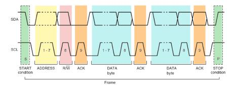
Figure 13-1: I2C writes access with 7-bit address
