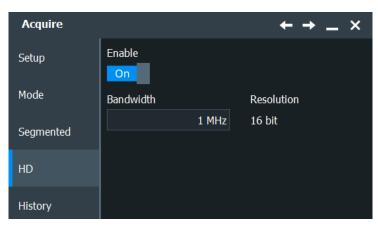
Figure 5-5: Setting the instrument into high definition mode
