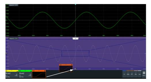
The diagram is converted into an XY-diagram.
