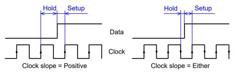
If at least one of the setup/hold measurements is selected, more settings appear to specify the measurement.
