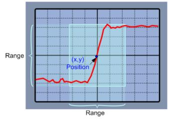
Figure 7-2: Numeric zoom using position and range
