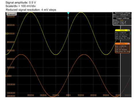
Figure 5-2: Traditional setup of multiple waveforms in one diagram: reduced resolution
