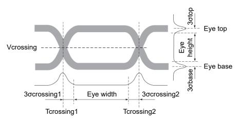
Figure 8-10: Basic eye diagram characteristics
