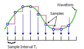
The digital ADC samples are processed according to the acquisition settings. The result is a waveform record that contains **waveform samples** and is stored in the **waveform memory**. The waveform samples are displayed on the screen and build up the waveform.
