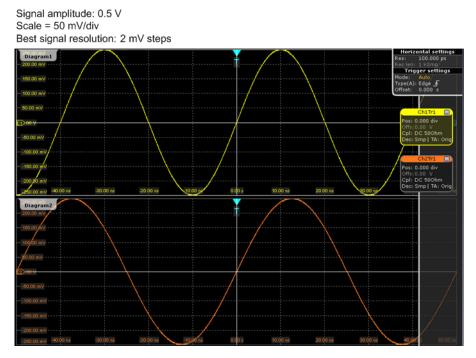
Figure 5-3: R&S RTO setup of multiple waveforms in separate diagrams: best resolution
