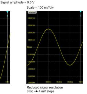
Figure 5-1: Input range and resolution of the ADC
