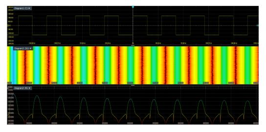
A spectrogram shows how the spectral density of a signal varies over time. The x-axis shows the frequency, the y-axis shows the time. A third dimension, the power level, is indicated by different colors. Thus you can see how the strength of the signal varies over time for different frequencies.
