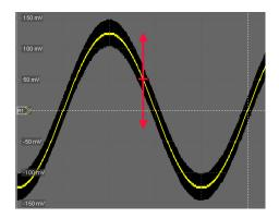
Figure 10-3: Waveform mask with vertical width = 0.5 div
