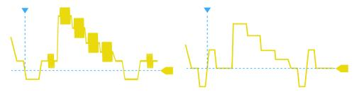
Figure 6-3: Bi-level (left) and tri-level (right) sync pulses
