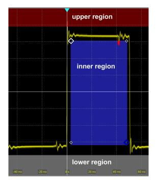
Alternatively, you can set the corner points on the touch screen and adjust the values in the "Mask Definition" tab.
