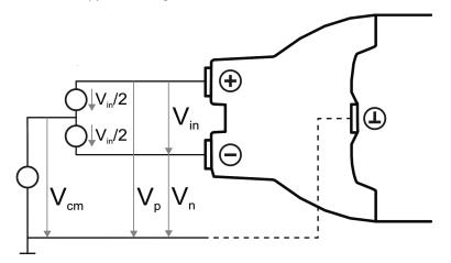
Multiple input voltages can be defined for a differential probe:
