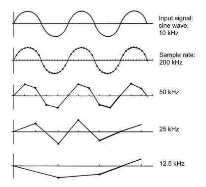
Figure 5-4: Waveforms acquired with different sample rates
