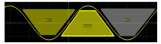
Figure 6-4: Indication of trigger zones
