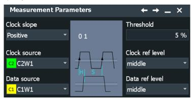
"Clock slope" Sets the edge of the clock from which the setup and hold times are measured: positive, negative, or either of them. If "Either" is selected, the clock edges next to the data edge are considered regardless of the clock slope.
